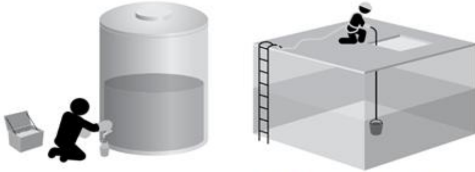
Sampling before water tank cleaning & disinfection
