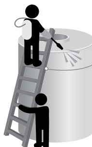
Spraying disin- fectant on Non- Man-Entry Tank internal surfaces
