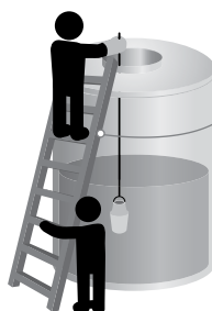
Sampling from Tanks with flushing valve
